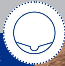
If a sewer shows damage only in the invert or crown area, a full renovation does not always make economic sense. For accessible sewers, pipe-segment lining is frequently used as a renovation technique.
